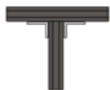
Double Corner bracket FFL 250-400mm
