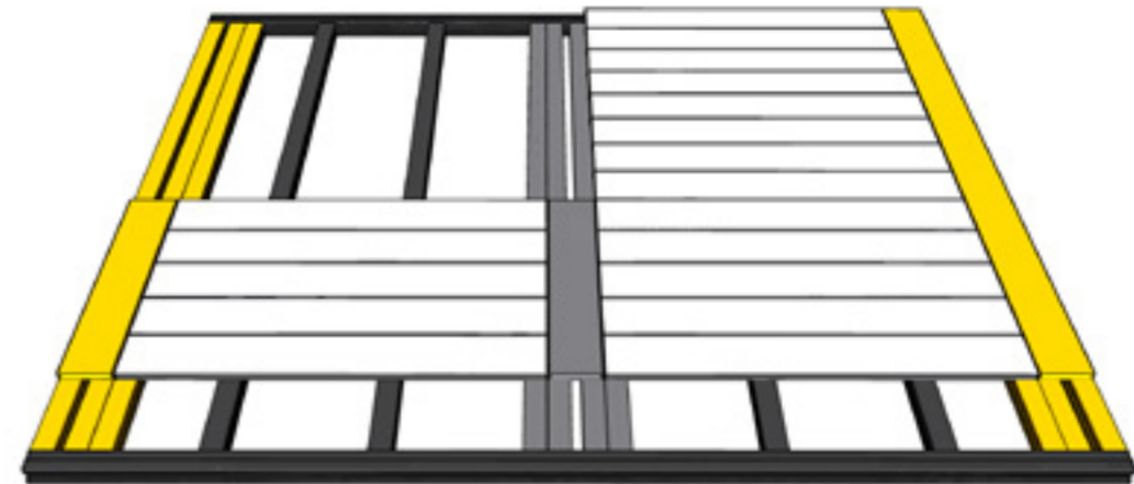
Picture Frame & Breakerboard using 2x additional joists
