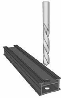
Predrill 28Profile (Max 8mm diameter hole)
