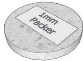
Insulating packer or similar to provide barrier between concrete and aluminium bracket must be used
